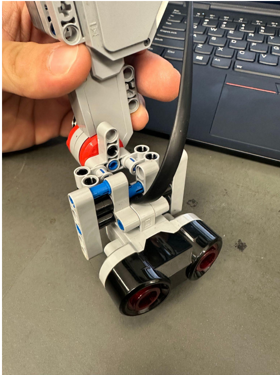
Image C.10 Top Of Front US Sensor Cable View
